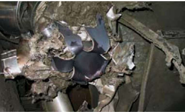
An exploded pipe inside the Brunsbüttel nuclear reactor in Germany - 14 Dec. 2001. © Greenpeace Germany
